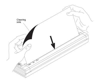
Figure 17. Inserting the cleaning cloth
